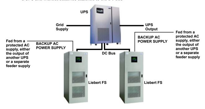
Figure 159 Multiple Liebert FS units operating with a UPS and without batteries attached to the DC bus
